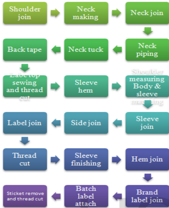
Fig 4: Layout of sewing for a T-shirt (scenario 3)
